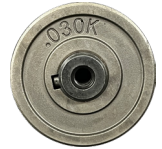
Wire diameter stamped on each side
